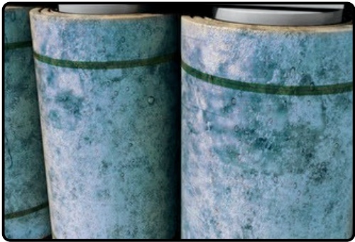
Degraded insulation paper due to moisture
